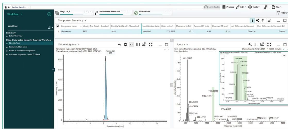
the FLP and shows their spectra and XIC integration that is used for quantification. Impurities are only included in this list if they are above a specified detection threshold (e.g., 0.2% relative intensity for  $m/z$  lower than the FLP and 0.3% relative intensity for  $m/z$  above the FLP in this case). To avoid double-counting, this list excludes anything chromatographically resolved from the FLP or present in the component list as a named impurity.
