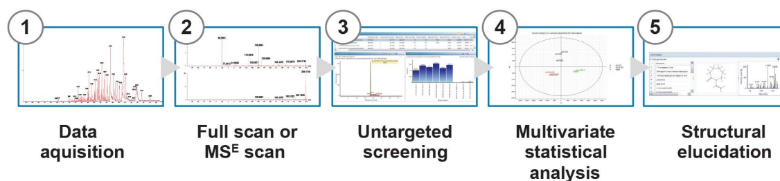
Figure 1. The analytical approach used for the analysis of virgin vs. recycled plastics, and the determination of chemical markers responsible for differences.
