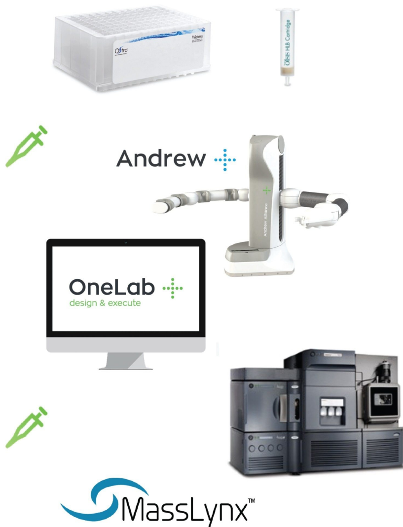
Figure 1. Graphical illustration of the automated SPE sample extraction and LC-MS analysis workflow using Oasis HLB SPE plates and cartridges and the Andrew+ Pipetting Robot configured with the Extraction+ Connected Device.
