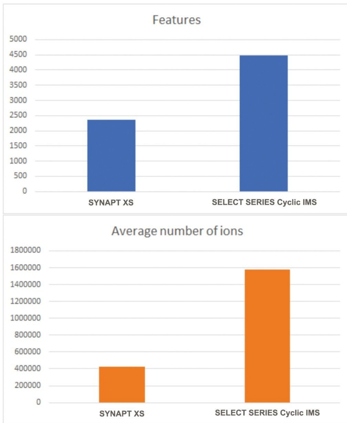
Figure 1. Comparison of the average number of peak-picked features and detected ions between the SYNAPT XS
