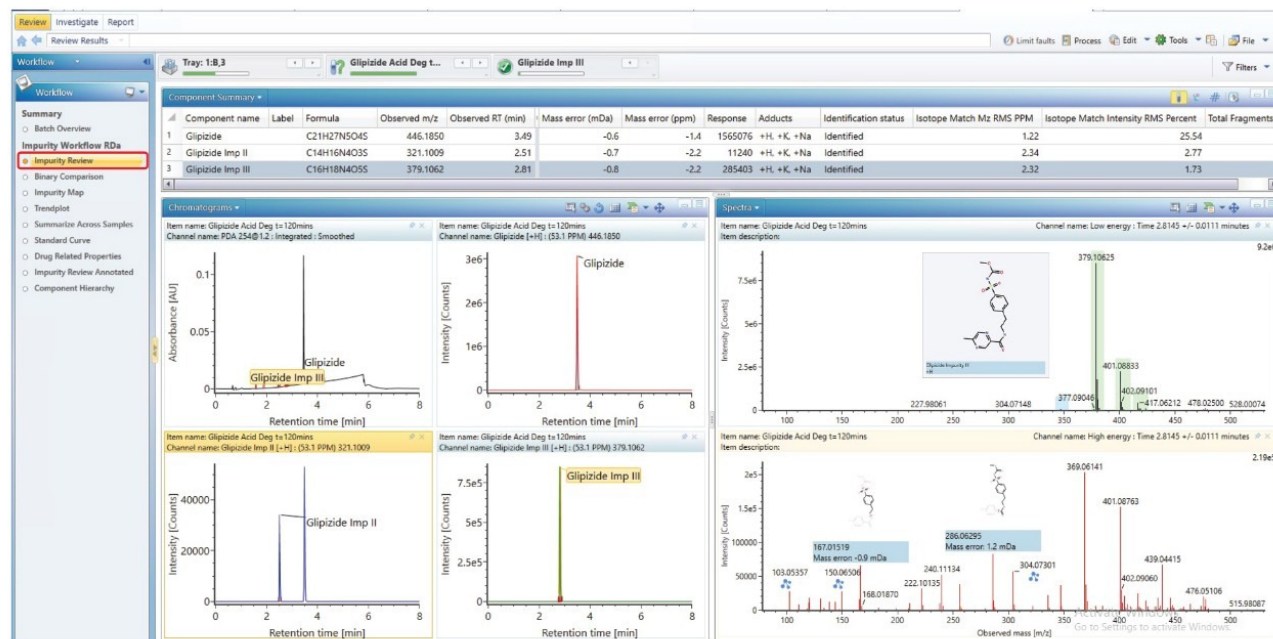
Figure 4. Low and high energy channels of glipizide Impurity III. Also shown are UV trace at 254 nm, and XIC's for API, impurity II and impurity III.
