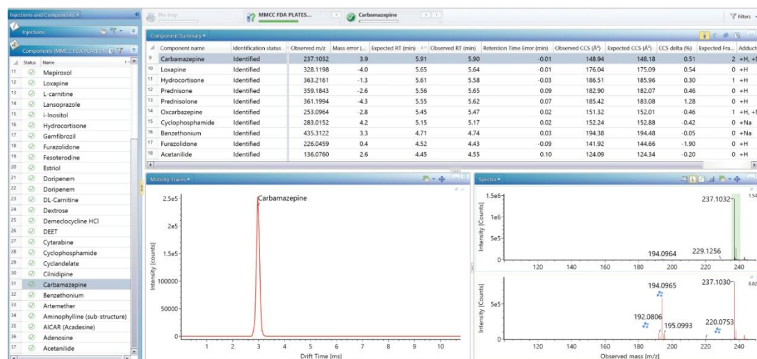
Figure 3. Post-acquisition processing workflow filtered detection results (identified count 37) for screening against FDA approved drug small molecule library, applied tolerance t_r 0.1 min, and mass accuracy \pm 5 pm and \Delta CCS <2%.
