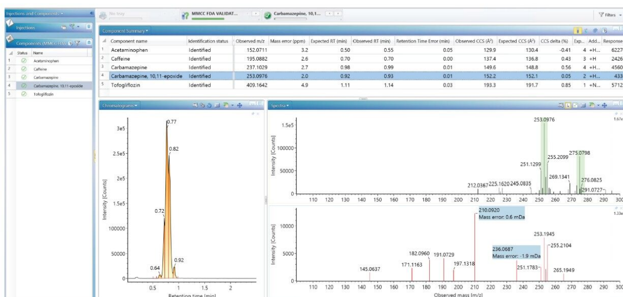
Figure 2. Detection results (identified count 5) for screening against fast gradient FDA small molecule library, applied t_r tolerance 0.1 min, and mass accuracy +/-5 ppm.
