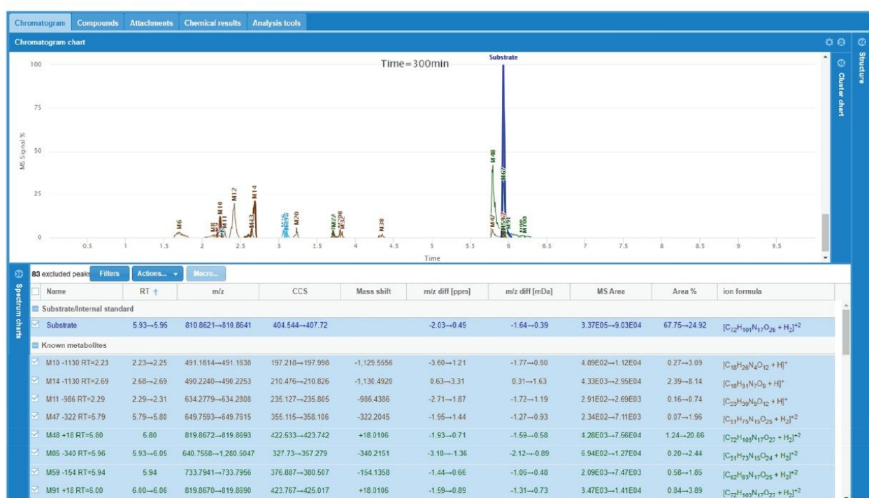
Figure 2. WebMetabase display of daptomycin incubation at 300 min. The top chromatogram is an overview of the substrate and major metabolites. The bottom table is a data summary for each observed peak.
