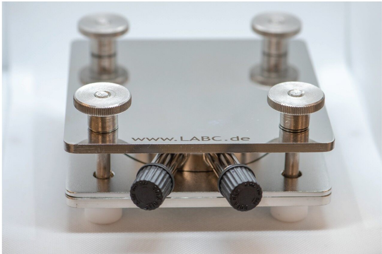
Figure 2. Photograph of the Siegwerk (Sieg-Mi-Flex) migration cell system (LABC-Labortechnik GmbH) used to perform single-sided migration study.
