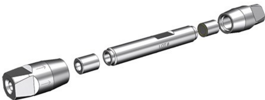
Figure 1. Explosion view of BioResolve SCX mAb Column hardware.
