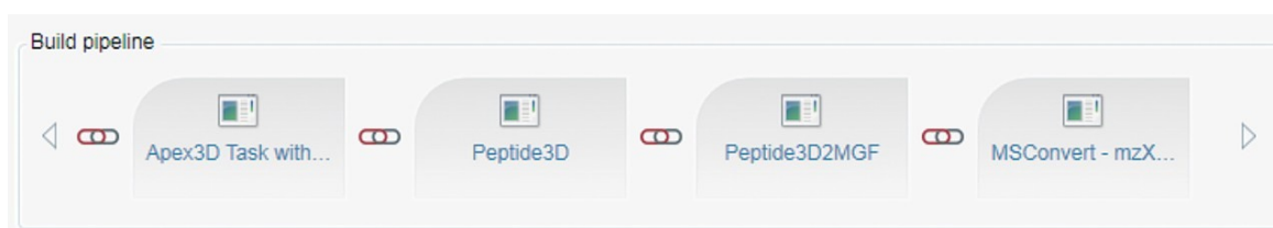
Figure 1. A Symphony pipeline example that chains 3D peak detection (Apex3D), deconvolution and deisotoping (Peptide3D), conversion to mgf, and subsequent MSConvert data conversion from mgf to mzML.
