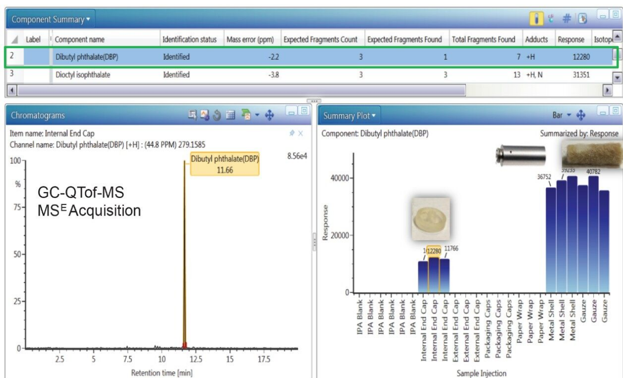
Figure 2. Identification of dibutyl phthalate (DBP) in the internal end cap, metal shell, and gauze using GC-QToF-MS.
