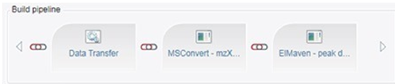
Figure 2. Symphony pipeline chains Robocopy data transfer followed by MSconvert, raw to mzXML data conversion and EIMaven peak detection, integration, annotation and upload.
