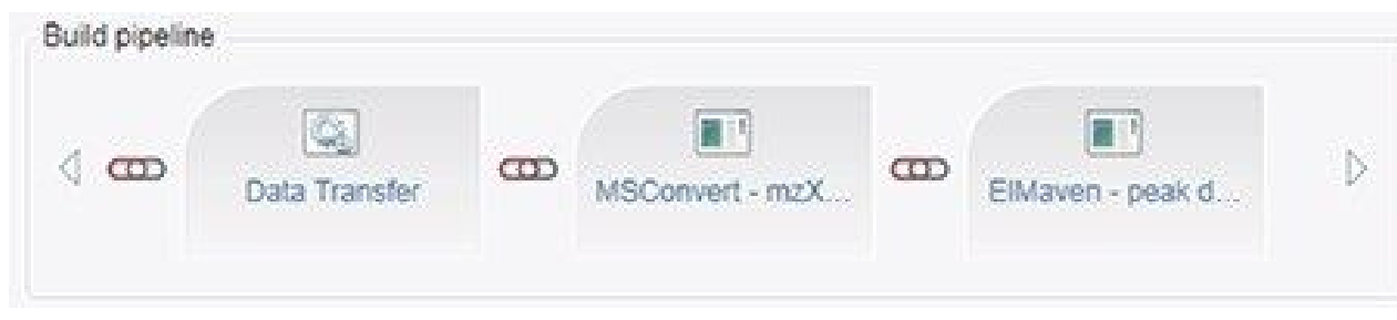
Figure 2. Symphony pipeline chains Robocopy data transfer followed by MSconvert, raw to mzXML data conversion and EIMaven peak detection, integration, annotation and upload.
