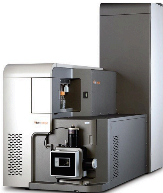
Figure 1. The Vion IMS QToF Mass Spectrometer – operated by workflow-driven, compliant-ready UNIFI Scientific Information System – provides a single platform for instrument control, data processing, and reporting.
