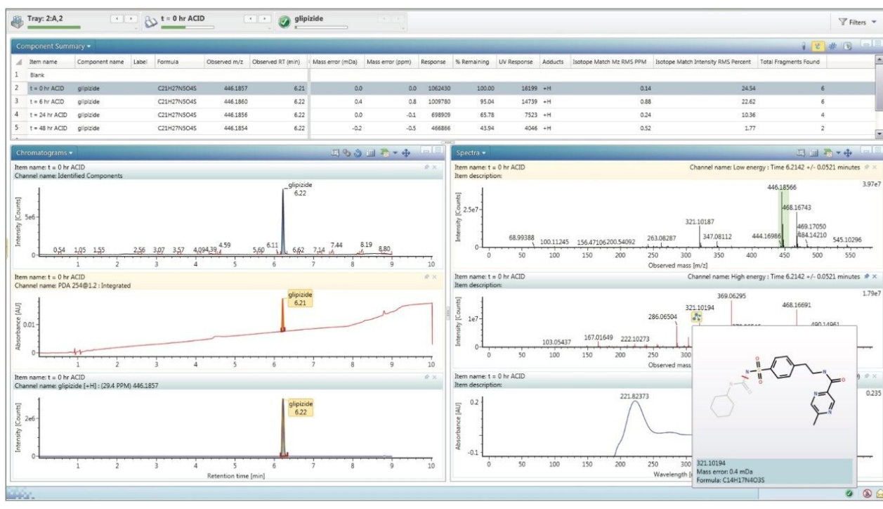
Figure 3. Low and high energy ( MS^E ) spectra and UV plot reported. The fragment ions are automatically assigned based on the structure (.mol file) of the API.
