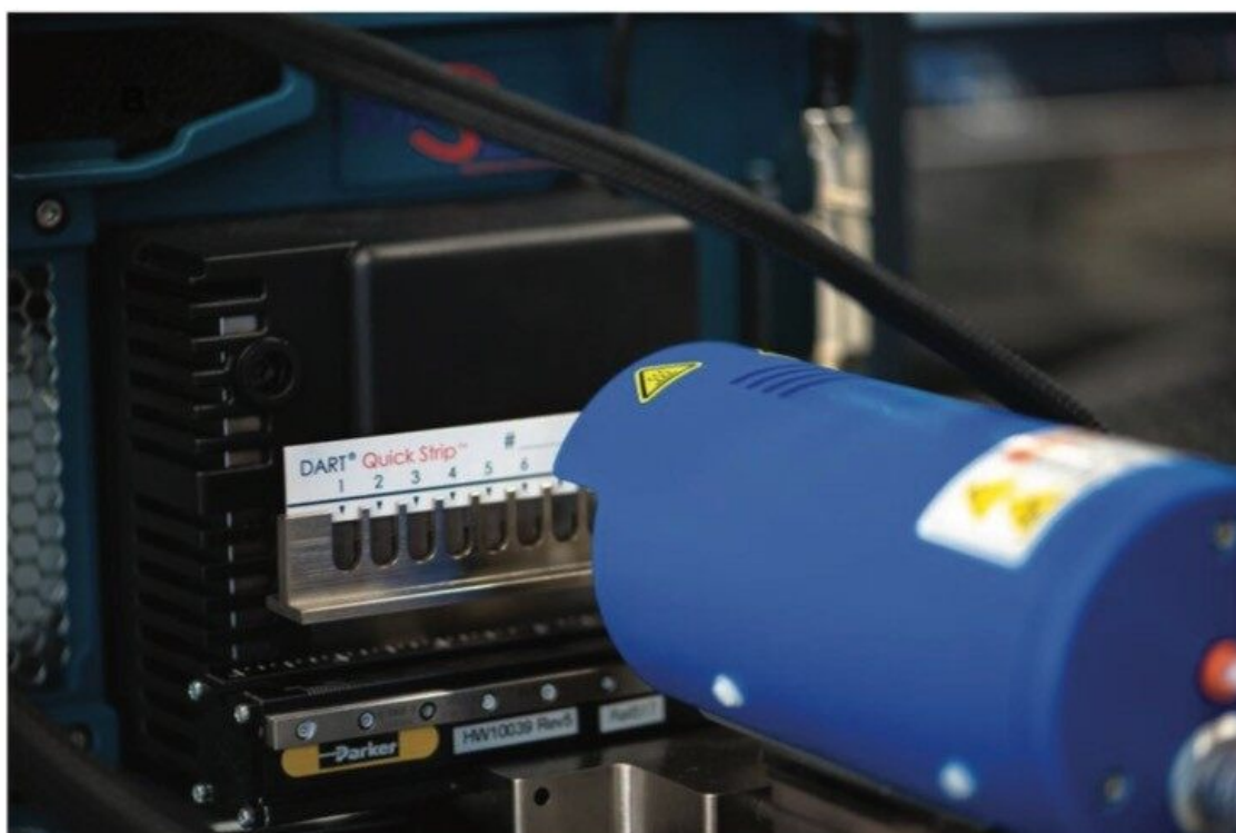
Figure 2. A. QuickStrip card used for sampling, B. automated multi-sample analysis.
