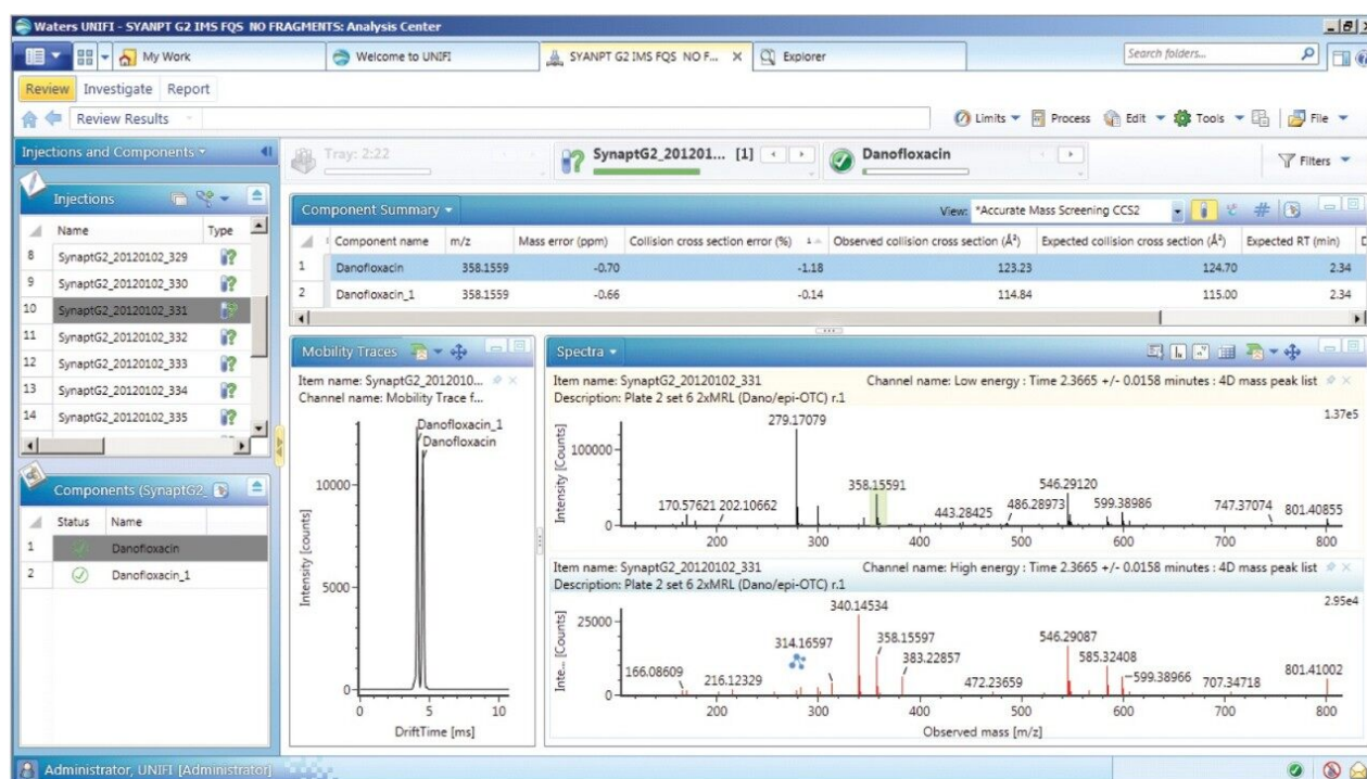
Figure 7. Identification of two danofloxacin protomers identified in porcine extract, where no ion mobility resolution spectral cleanup has been selected. Precursor ion and fragmentation with matrix background ions are shown for danofloxacin protomer, expected CCS 124.7 Å².
