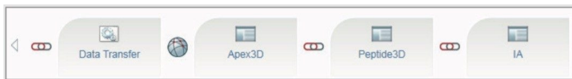
Figure 2. The Symphony task sequence for data processing. RAW files were copied from the instrument-linked PC over a local network to a second PC where Apex 3D, Peptide3D, and IA were executed in sequence.
