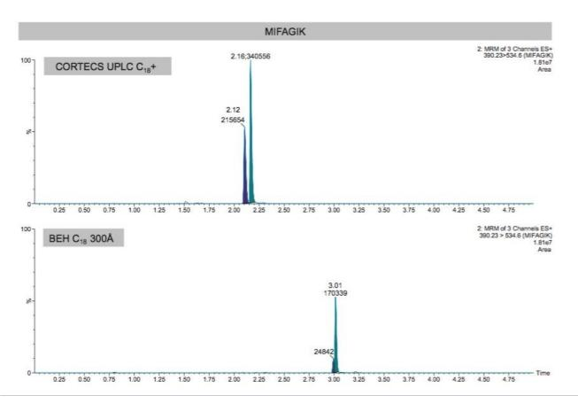
Figure 4. Representative chromatograms demonstrating improved specificity and resolution from interference (RT 2.12) using the CORTECS UPLC C<sub>18</sub>+ for the MIFAGIK (RT 2.16) cytochrome C tryptic peptide.
