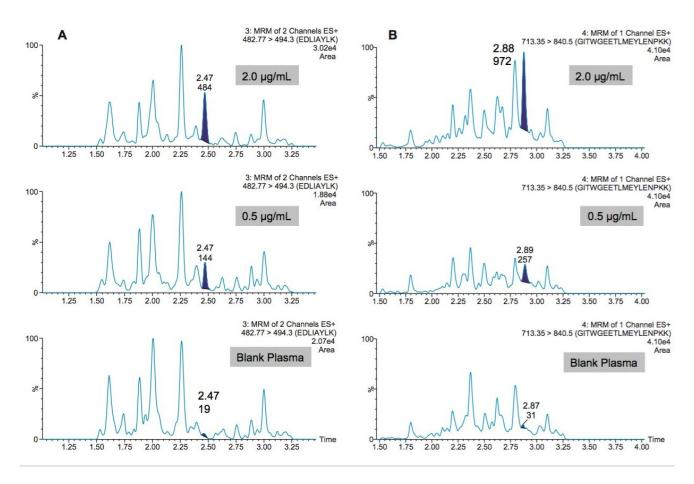
Figure 6. Chromatograms demonstrating sensitivity of the MIFA (A) and GITW (B) peptides, at the LOQ (2.0  $\mu g/mL$ ) and LOD (0.5  $\mu g/mL$ ), respectively.
