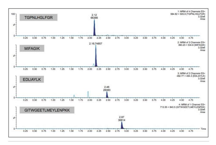
Figure 3. UPLC chromatographic separation of cytochrome C tryptic peptides (mid QC samples), using the CORTECS UPLC  $C_{18}$ + 90Å, 1.6  $\mu$ m, 2.1 mm  $\times$  50 mm Column.
