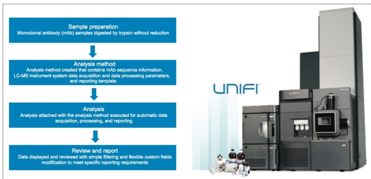
Figure 1. Disulfide bond mapping using the Waters Biopharmaceutical Platform Solution with UNIFI. The workflow encompasses automated UPLC-MS E data acquisition, processing, and reporting.
