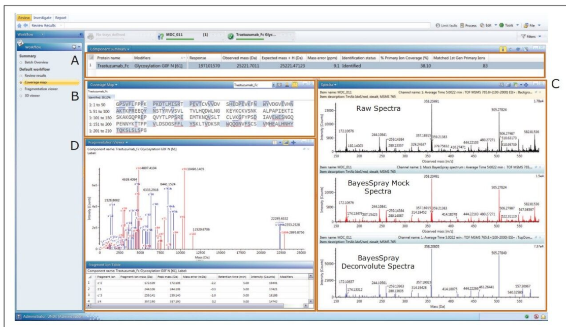
Figure 4. Example of infusion top-down analysis of the trastuzumab Fc/2 subunits with targeted MS-MS data acquisition using ETD fragmentation.
