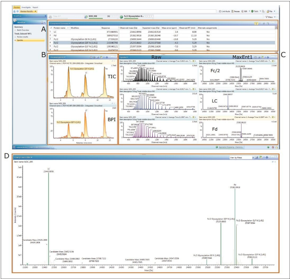
Figure 2. Trastuzumab (T-mab) subunit LC-MS analysis with MaxEnt1 deconvolution processing and UNIFI intact MS analysis workflow.
