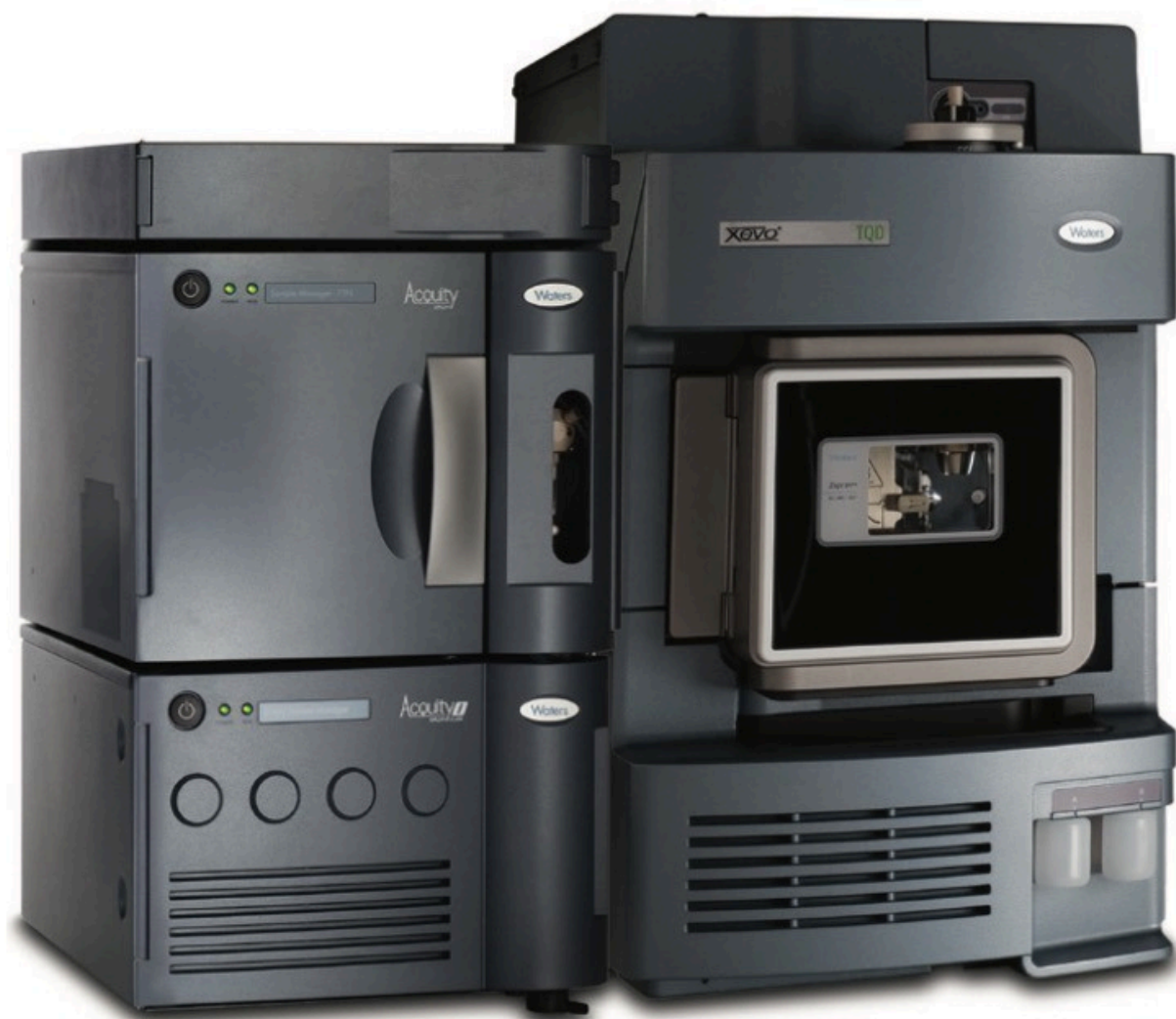
Figure 1. The ACQUITY UPLC I-Class and Xevo TQD.
