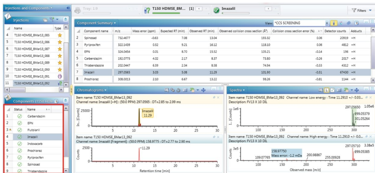
Figure 5. IonKey/MS System ion mobility results for EU RL proficiency test FV-13 pesticide residue screen. A data filter comprising 2% CCS error and threshold response was applied with nine observations made (highlighted in red).
