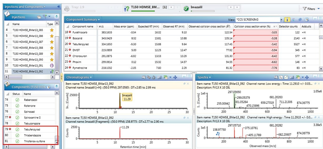
Figure 4. ionKey/MS System ion mobility results for EU RL proficiency test FV-13 pesticide residue screen using an accurate mass measurement tolerance of 10 ppm and CCS tolerance of 10% for the target residues. To determine the unknown iKey Separation Device retention times, a 30 min retention time window was applied, 81 observations made (highlighted in red).
