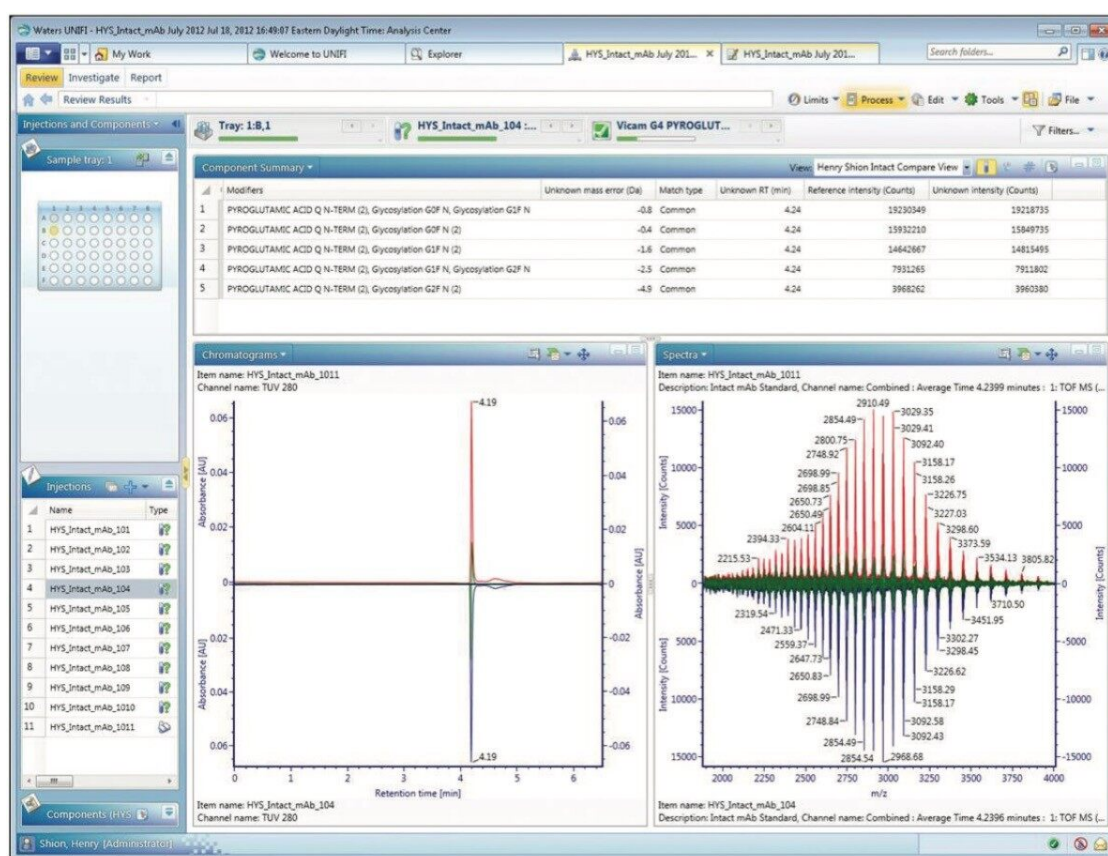
Figure 3. UNIFI's review panel (compare mode) displays automatically processed experiment results, with a focus on identifying similarities and differences between a reference sample and unknown samples.
