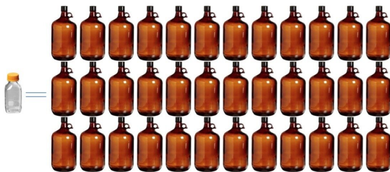
Figure 9. Comparison of relative solvent consumption of ionKey running at 7 \mu\text{L}/\text{min} flow rate vs. analytical scale chromatography running at 1 mL/min flow rate is displayed. The figure shows that consuming 1 L solvent on the ionKey/MS System running continuously at 7 \mu\text{L}/\text{min} for 99 days or 35,700 injections at 4 min run time, is equivalent to thirty six 1-gallon bottles using an analytical scale system.
