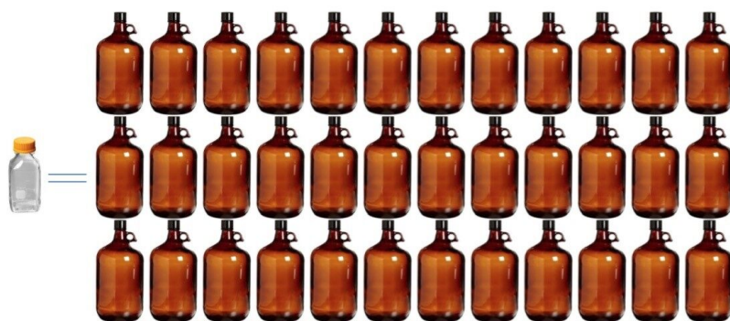
Figure 9. Comparison of relative solvent consumption of ionKey running at 7 \mu\text{L}/\text{min} flow rate vs. analytical scale chromatography running at 1 \text{mL}/\text{min} flow rate is displayed. The figure shows that consuming 1 L solvent on the ionKey/MS System running continuously at 7 \mu\text{L}/\text{min} for 99 days or 35,700 injections at 4 min run time, is equivalent to thirty six 1-gallon bottles using an analytical scale system.
