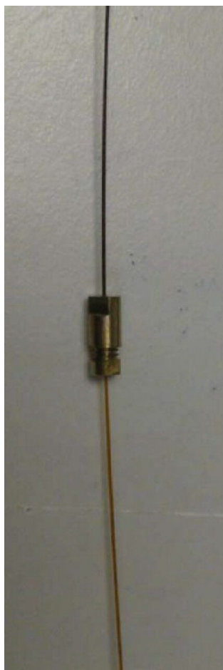
Figure 15 SilTite \mu -Union connect column and retention gap.
