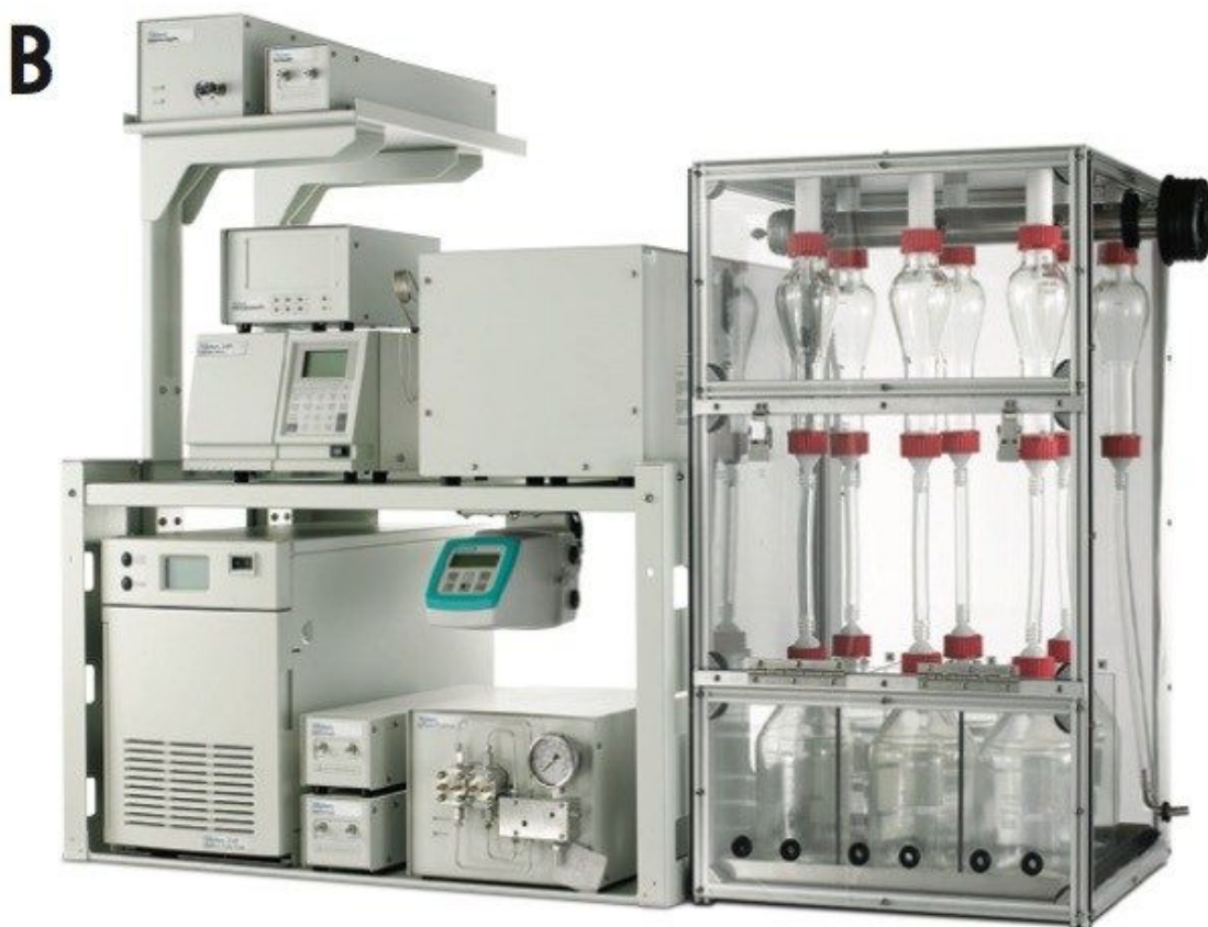
Figure 1. MV-10 ASFE (A) and Prep 80q SFC (B) systems used to extract and purify the vanillin.
