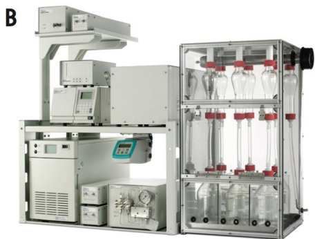
Figure 1. MV-10 ASFE (A) and Prep 80q SFC (B) systems used to extract and purify the vanillin.
