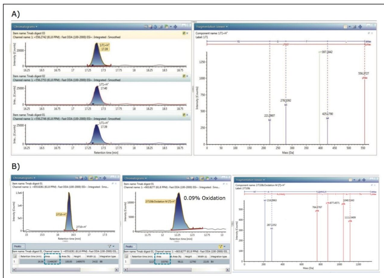
Figure 2. Peptides present at low abundance were identified with high confidence using the FastDDA method. A) LeuEnk was identified in all three injections at 0.1% level (25 fmol load on column). XIC of each run is shown on the left and the annotated MS/MS spectrum is shown on the right. B) XICs of non-modified 2:T10 and oxidized 2:T10, with peak areas shown in the table below. The annotated MS/MS spectrum of oxidized 2:T10 is displayed in the Fragmentation Viewer.
