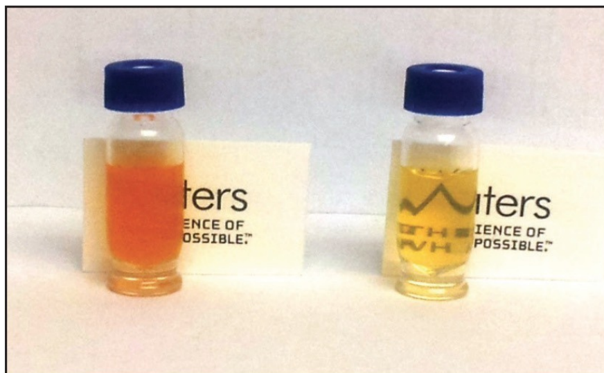
Figure 2. SPE cleanup for LC-MS; vial on left shows a chili powder sample prepared with no dSPE cleanup, vial on right shows a sample prepared with dSPE cleanup.
