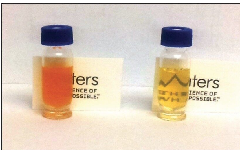
Figure 2. SPE cleanup for LC-MS; vial on left shows a chili powder sample prepared with no dSPE cleanup, vial on right shows a sample prepared with dSPE cleanup.
