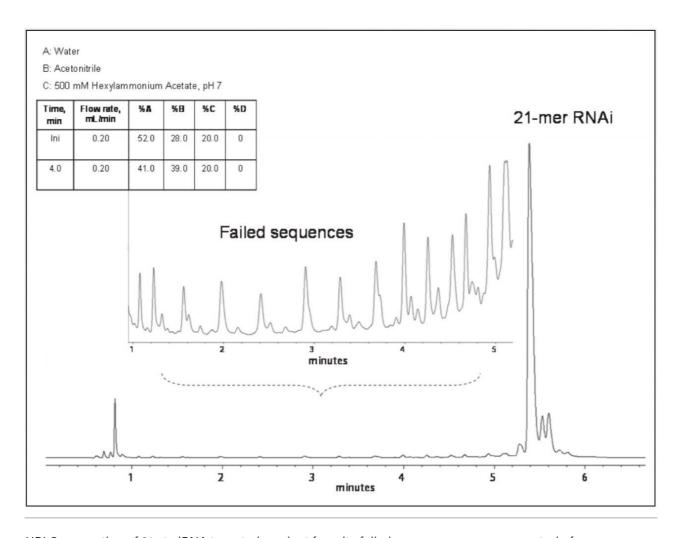
UPLC separation of 21 nt siRNA targeted product from its failed sequences serves as control of oligonucleotides synthetic quality. The Auto•Blend function of the ACQUITY UPLC H-Class Bio System allows an automatic mixing of three solvents resulting in fast and accurate analysis procedure.
