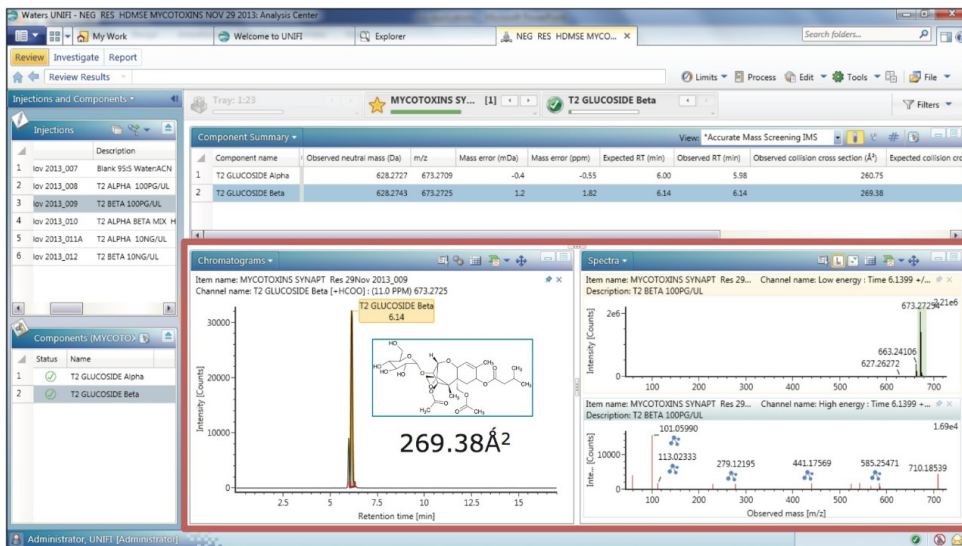
Figure 2. UNIFI Software screenshot showing CCS value for a masked mycotoxin compound T2 \beta -glucoside together with the corresponding exact mass precursor ion and ion mobility product ion spectra.
