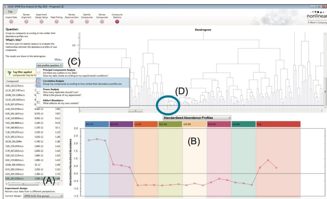
Figure 5. Accessing and using the correlation analysis within Progenesis Q1 (C) enables the user to extract further ions of interest that follow a similar profile to a selected marker (B).
