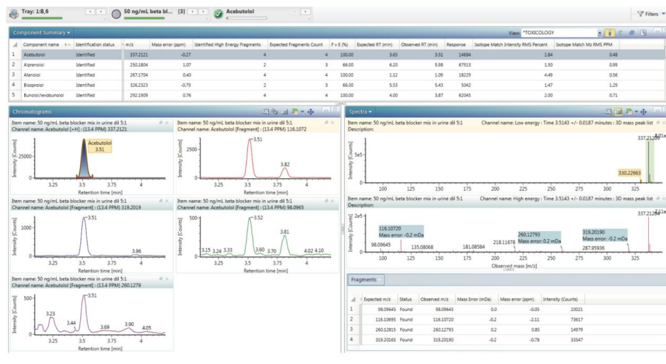
Figure 2. Details for a 50 ng/mL spiked urine sample. The Component Summary shows details for the first five analytes present in alphabetical order. The F v E (%) column displays the number of found vs number of expected fragments, expressed as a percentage. The Isotope Match Intensity RMS Percent and Isotope Match Mz RMS PPM indicate the degree of matching between the theoretical isotopic pattern and the observed pattern for the precursor ion cluster. The chromatogram's window contains the extracted mass chromatograms for the selected precursor i.e., acebutolol ( m/z 337.212) and fragment ions ( m/z 116, 319, 98, and 260). The Spectra window displays the low collision energy (upper spectrum) and high collision energy (lower spectrum) for acebutolol and the Fragments table shows each of the expected fragments for acebutolol.
