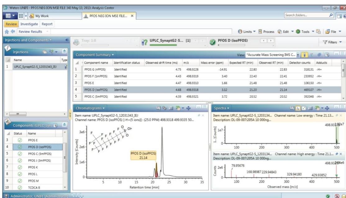
Figure 7. PFOS (D) (isoPFOS) isomer ion mobility precursor ion and characteristic fragmentation spectra, ion mobility resolved from isobaric interference TDCA (A), at retention time 21.14 mins.
