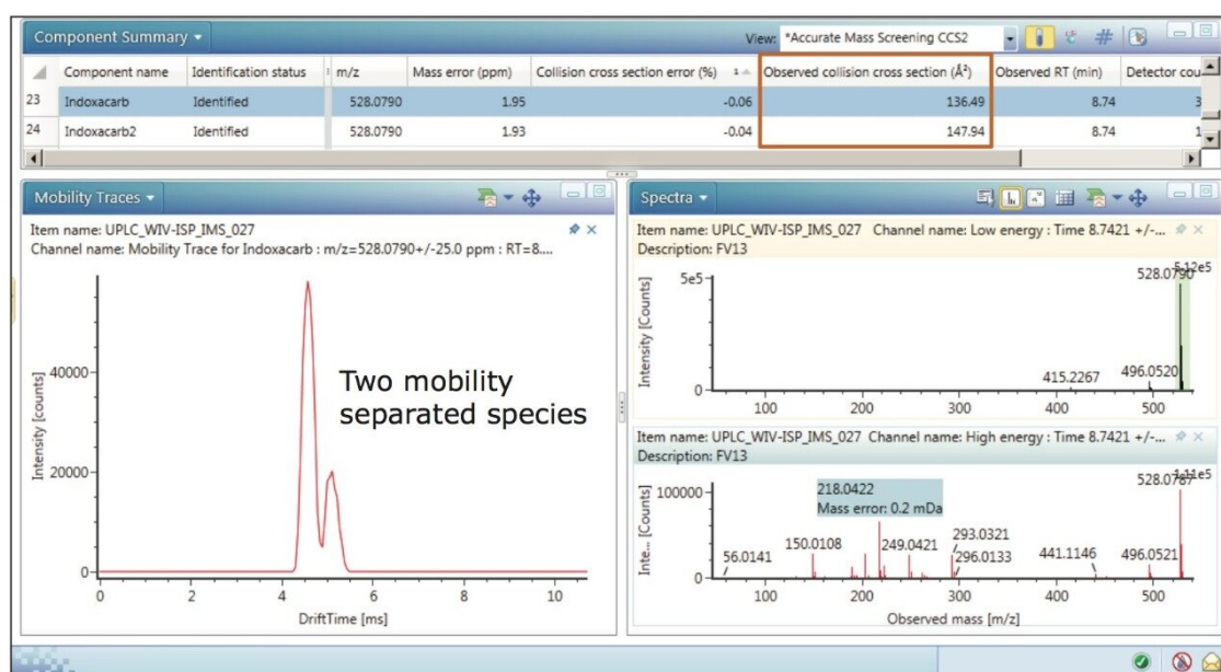
Figure 3. Mobility trace illustrating the observation of two protomers and corresponding CCS measurements of 136.49 Å 2 and 147.94 Å 2 , comprising the extracted mass chromatogram for indoxacarb observed in proficiency sample FV-13.
