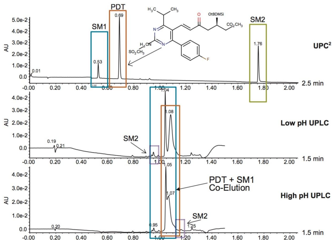
Figure 3. Chromatographic overlays at 298 nm of (A) ACQUITY UPC 2 , (B) UPLC low pH, and (C) UPLC high pH results for time point 5 (T 5 = 6hrs).
