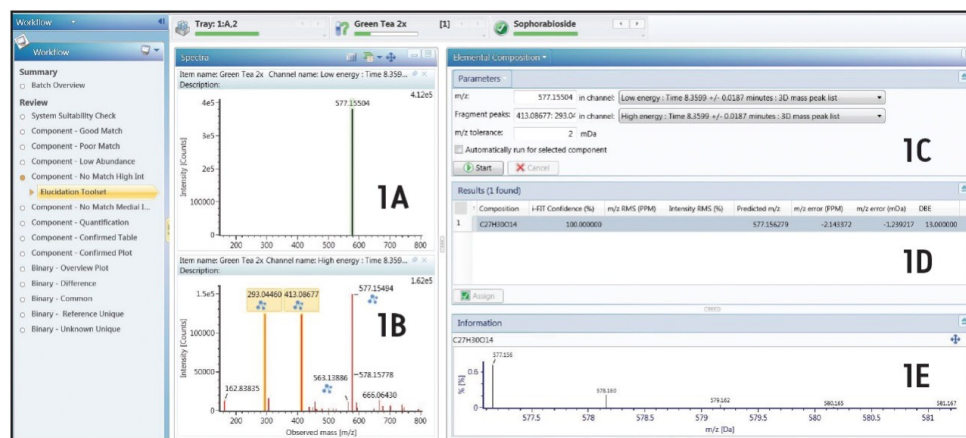
Figure 1. The process of an unknown component's elemental composition determination. 1A: Low collision energy mass spectrum of the unknown component. 1B: High collision energy mass spectrum of the unknown component. 1C: Settings for elemental composition search. 1D: Search results of the unknown component's elemental composition. 1E: Isotope distribution plot for the unknown sample.
