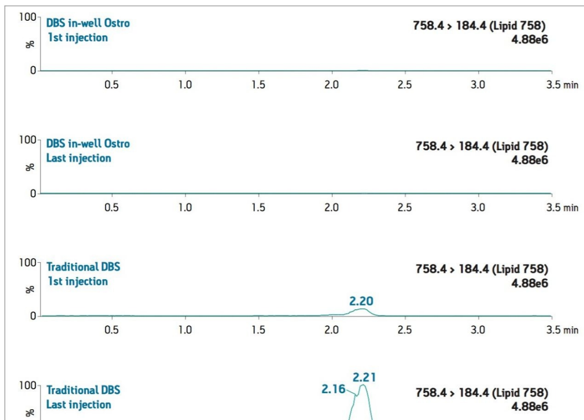
Figure 5. Chromatograms of the MRM transition 758>184 to demonstrate build-up of an individual PL over subsequent injections using traditional DBS and DBS extracted in-well using the Ostro Pass-through Plate. A gradient from 25 99.5% B in 2 minutes was used followed by a 1-minute hold at high organic.
