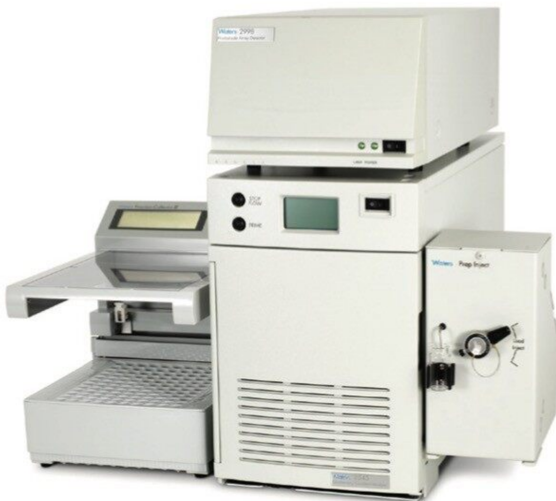
Figure 2. Waters Prep 150 LC System.
