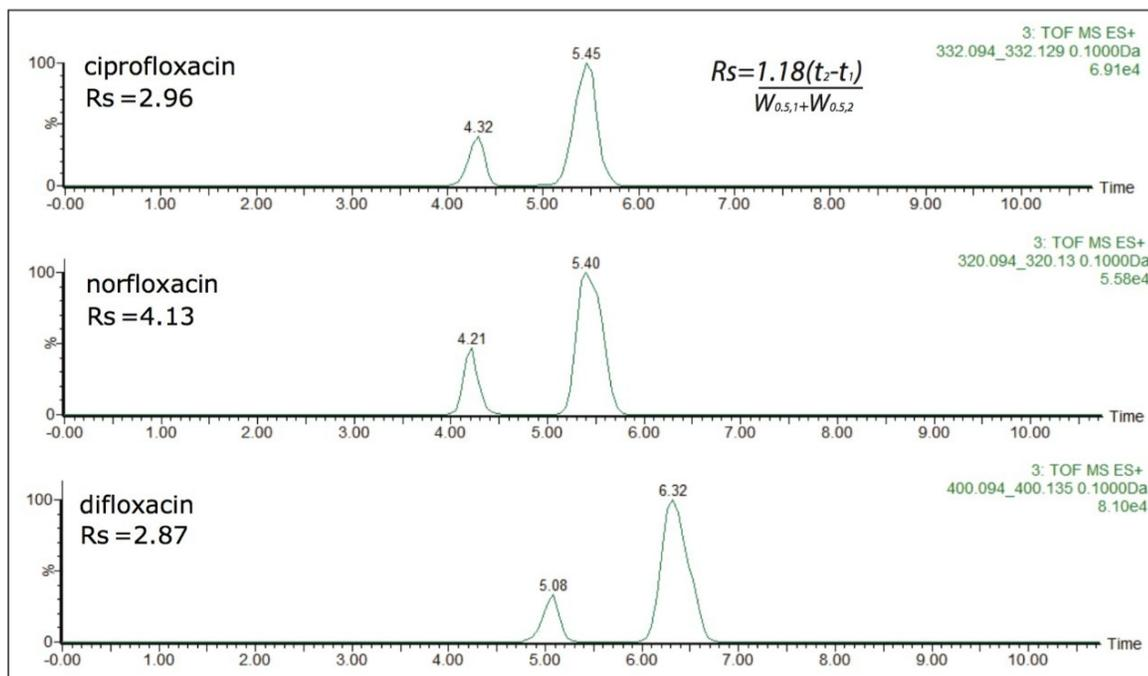
Figure 9. Illustration of ion mobility separation achieved for fluoroquinolone antibiotics using UPLC IMS with N<sub>2</sub> drift gas. Peak-to-peak resolution was calculated at half height using the equation shown.
