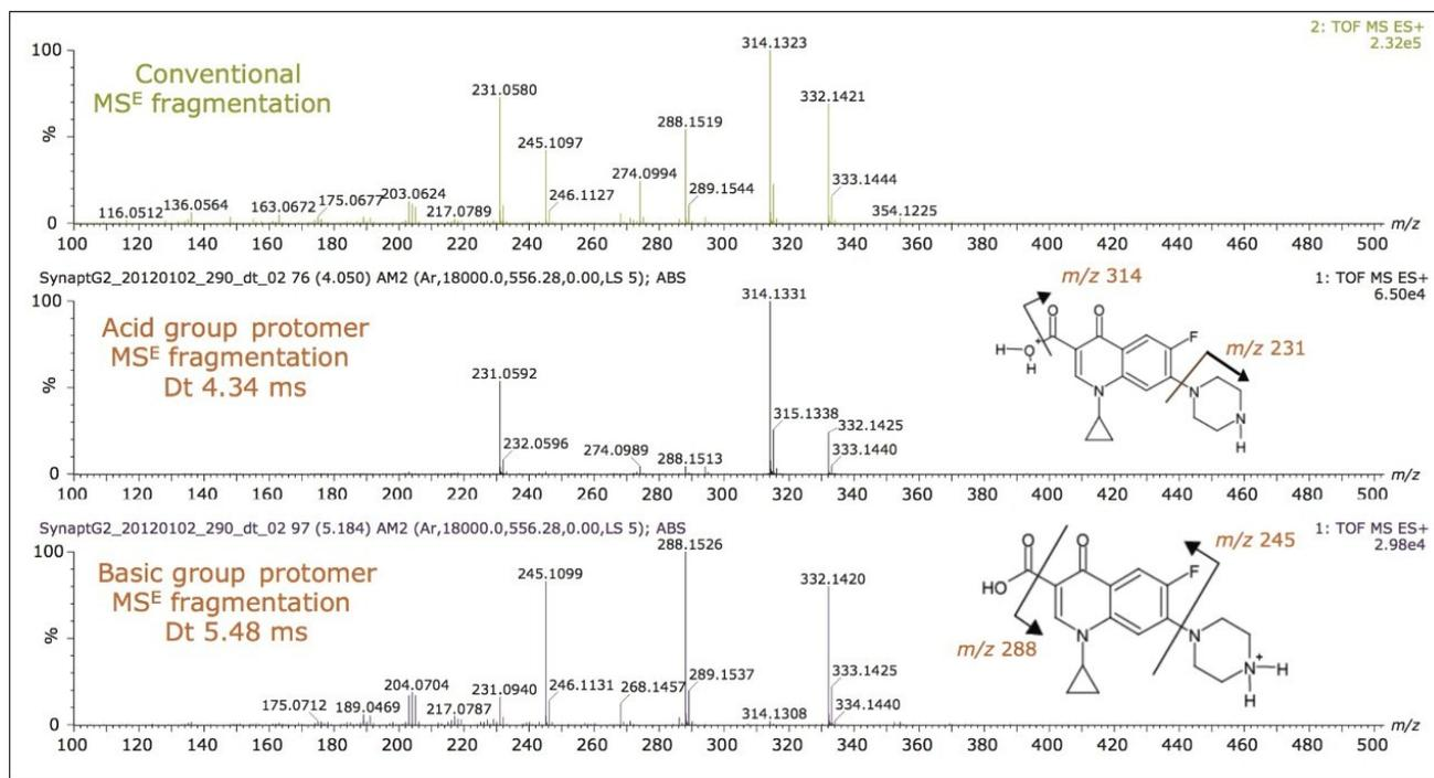
Figure 7. Conventional ciprofloxacin ( $m/z$  332) MS accurate mass fragmentation spectrum and individual accurate mass fragmentation spectra for ciprofloxacin protomers comprising the conventional fragmentation spectrum.
