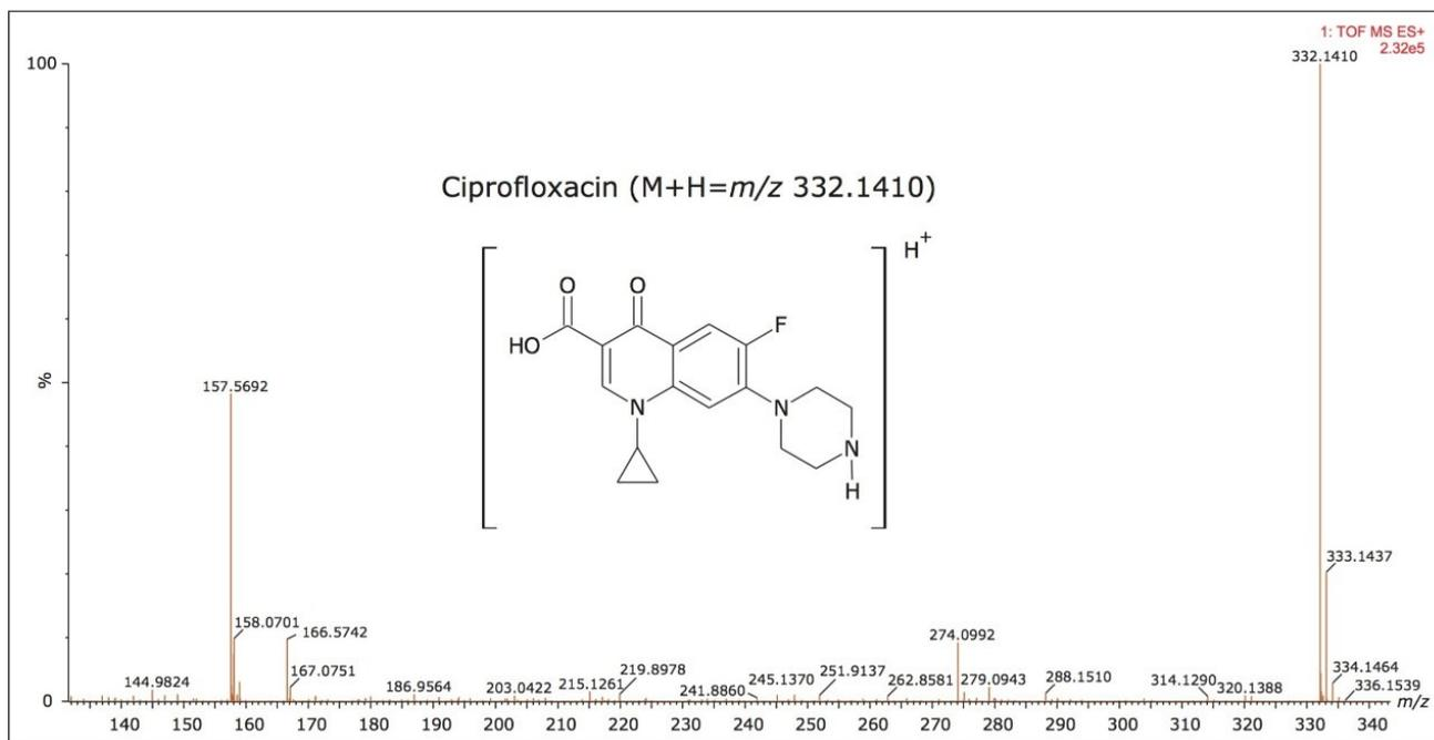
Figure 4. Conventional UPLC HDMS<sup>E</sup> accurate mass precursor ion spectrum obtained for the standard fluoroquinolone ciprofloxacin at retention time of 2.19 minutes, illustrated within MassLynx.
