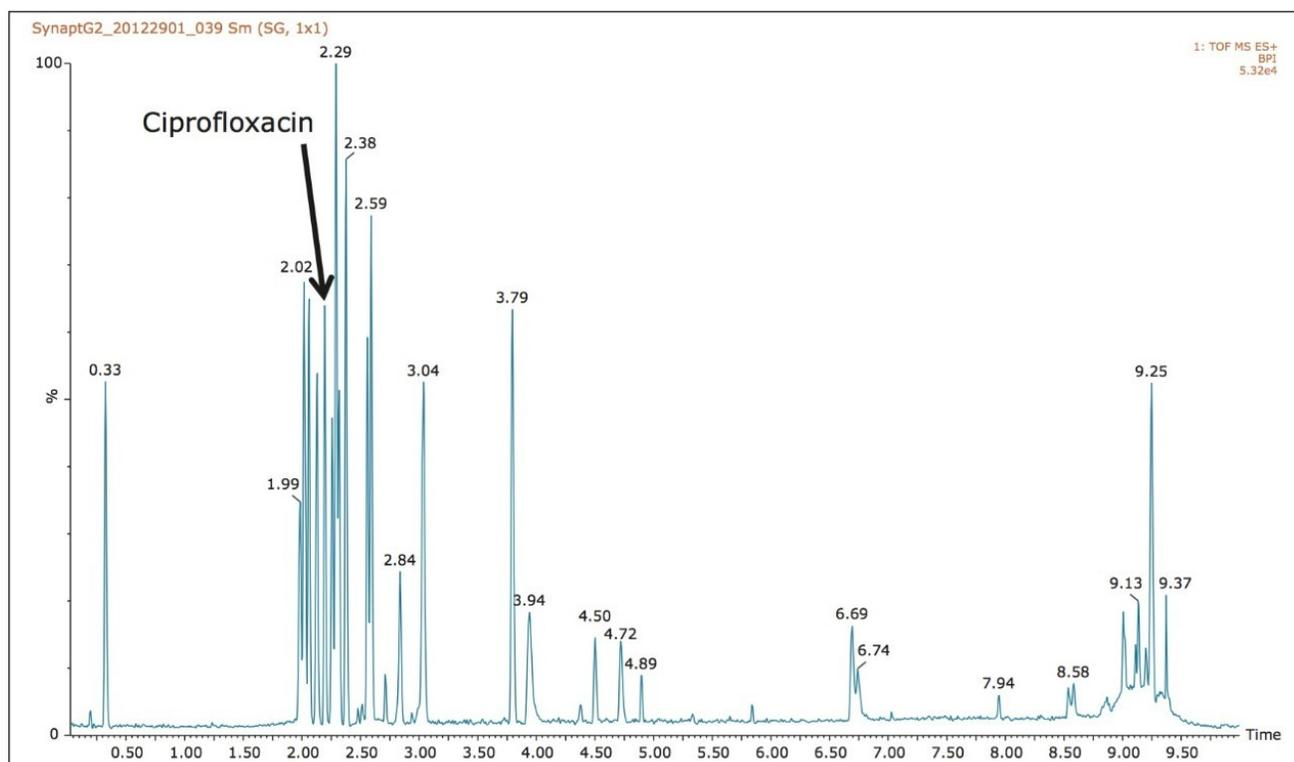
Figure 3. UPLC HDMS<sup>E</sup> precursor base peak ion chromatogram for a mixture of 25 solvent standard antibiotic compounds.
