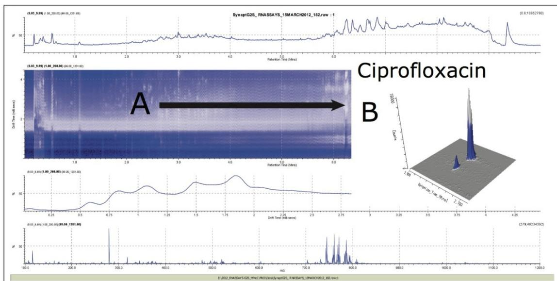
Figure 8. Illustration of matrix removal for ciprofloxacin in porcine extract, where the 3D display of
