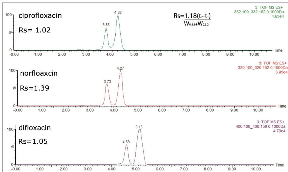
Figure 10. Illustration of ion mobility separation achieved for fluoroquinolone antibiotics using UPLC IMS with CO<sub>2</sub> drift gas. Peak-to-peak resolution was calculated at half height using the equation shown.
