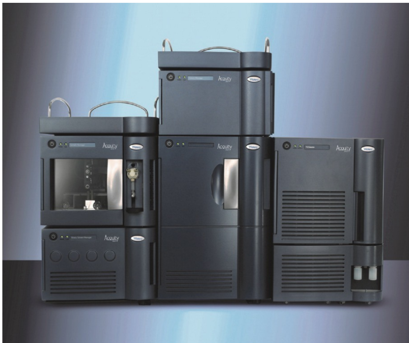
Figure 1. System configuration of a Waters ACQUITY UPLC coupled to a MassTrak Online SPE Analyzer and ACQUITY TQ Detector.
