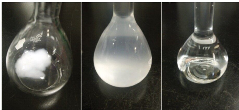
Figure 1. RHINOCORT AQUA (budesonide) nasal spray sample preparation. (a) RHINOCORT AQUA (budesonide) nasal spray formulation; (b) budesonide formulation in diluent; (c) budesonide sample after centrifugation.
