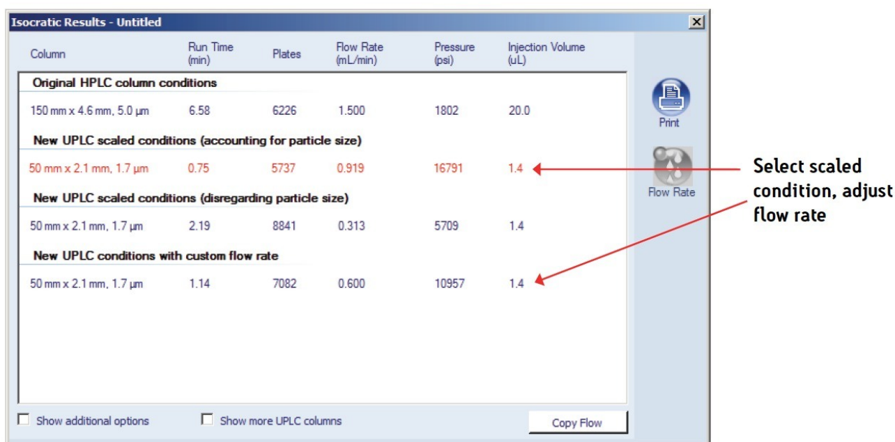
Figure 1. ACQUITY UPLC Columns Calculator result showing original and scaled conditions.
