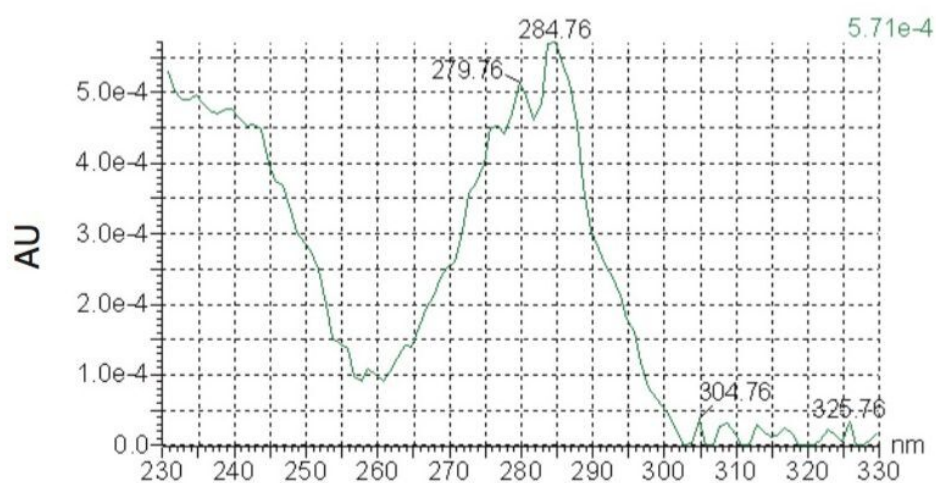
Figure 8. UV spectrum obtained from the incurred sample and the reference standard at 10 ng/g.
