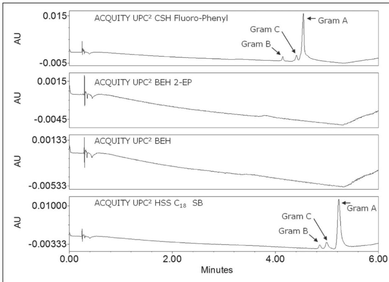
Figure 1. A variety of column chemistries were screened for chromatographic peak shape and retention of a gramicidin standard. All columns contained sub-2- $\mu\text{m}$  particles packed in 3.0 x 100 mm hardware. All separation conditions were MP A: CO<sub>2</sub>, MP B, 0.1% FA in MeOH, 2 mL/min, 3% to 25% B in 5 min.
