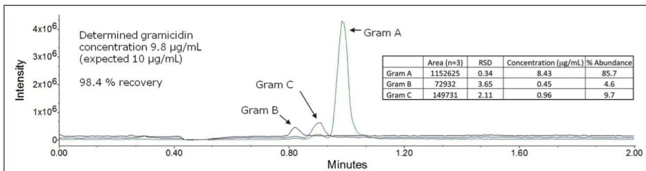
Figure 6. Overlay of selected ion chromatograms for gramicidin A, B, and C extracted from antibacterial ointment. Calculated RSD values for replicate analyses ( $N = 3$ ) are within acceptable values. Calculated abundances are in good agreement with literature reported values.<sup>1</sup>
