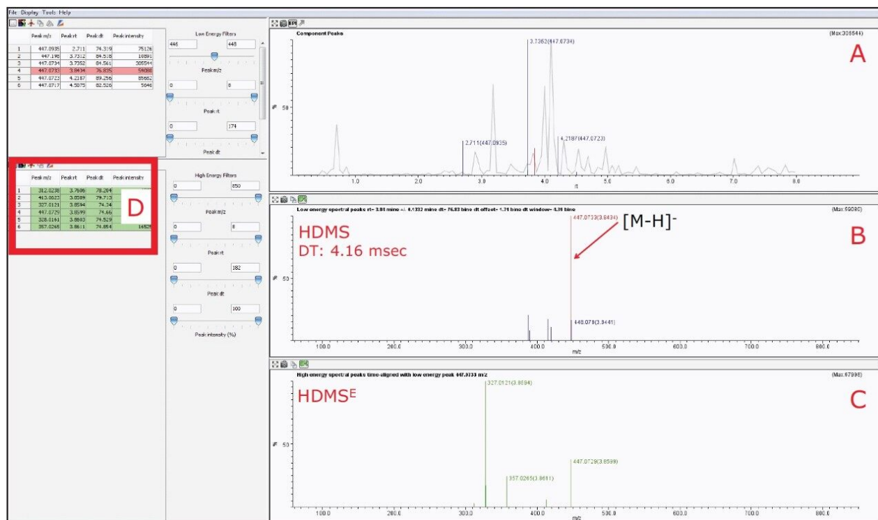
Figure 7. Orientin peak at 3.84 min with HDMS function activated. 7A. Chromatogram of peaks with 447.0927 m/z . 7B. Low energy mass spectrum (HDMS) with orientin peak selected (highlighted in red). 7C. High-energy mass spectrum (HDMS E ) of orientin peak. 7D. List of product ions present in the HDMS E spectrum.
